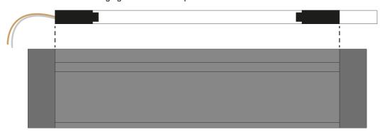
2. Using a PVC Conduit Cutter (or similar), cut the LR1238 TUBE to the required length of the recess, minus the length of the LEDCHAM + BLANK (as illustrated below).
